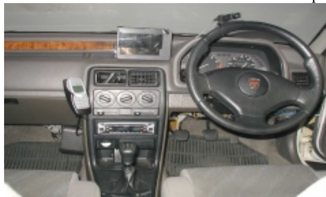
Figure 2 – Interior of driving simulator and hands-free phone
