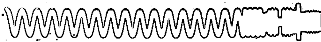
Figure 1. Simoco helical antenna.
