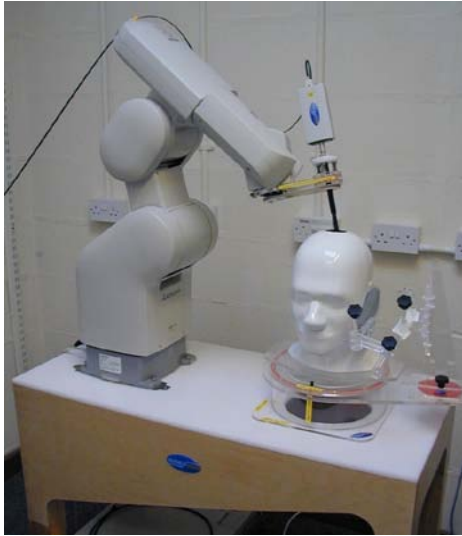
Figure 12: Robot arm, probe and head phantom
